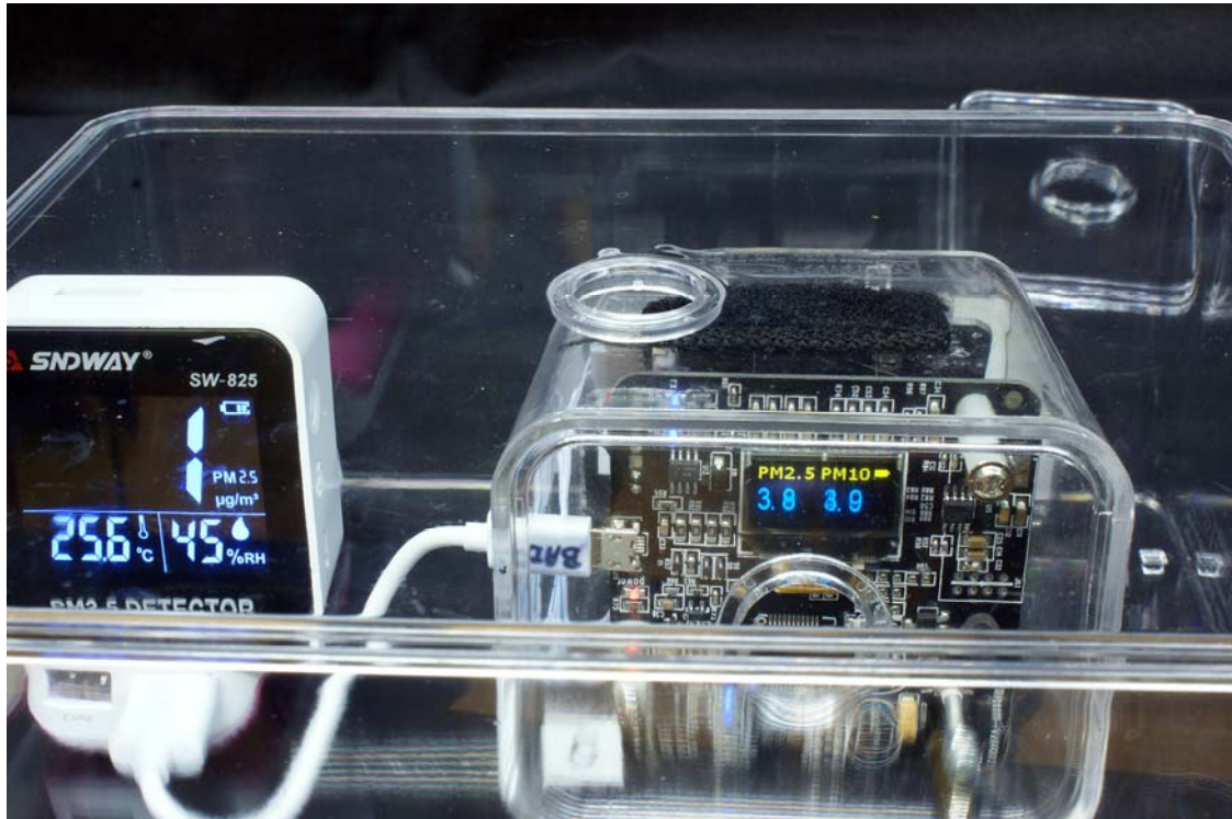
Fig. 15: Dry box: RH = 45%, PM2.5 = 3.8, PM10 = 3.9 \mu\text{g}/\text{m}^3
