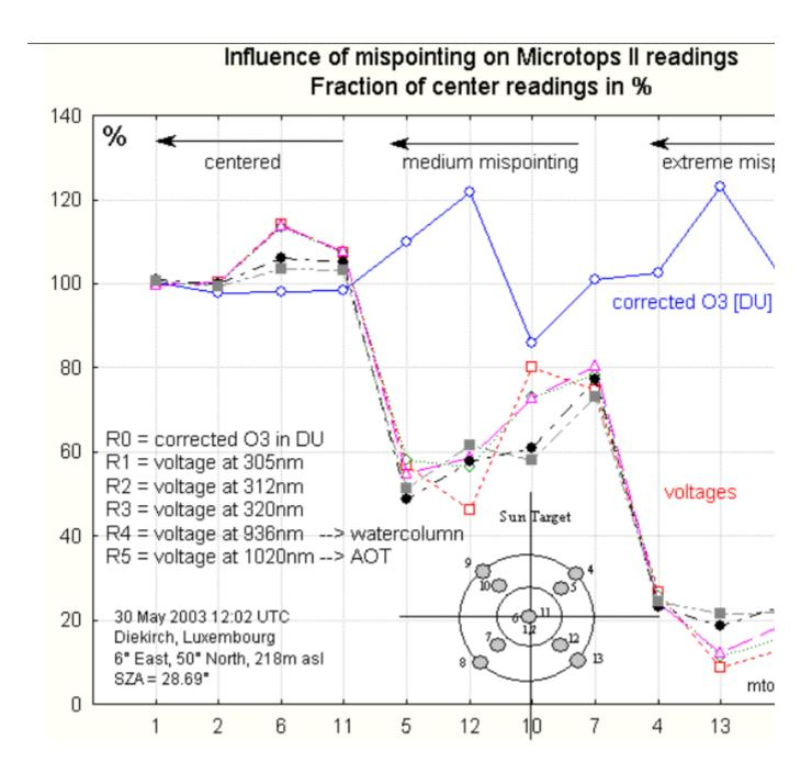
Ichoku [ref. 3] writes that the AOT error increases in exponential fashion with the deviation of the sun's image from the center; our data of the raw voltages (curve R5) confirm this: if we take the three readings labeled 1, 12 and 13, the distances (x) from the center are about 0, 2 and 3 with the corresponding percental errors (E) 0, 20 and 80.
