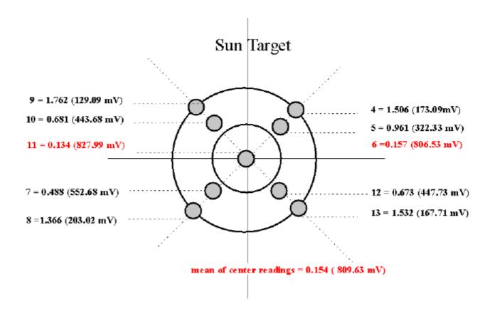
Conclusion: The AOT readings deviate extremely, such as to give unusable values if the sun disk is not correctly centered on the target. The voltages decrease with increasing pointing error for both diagonals; even if this decrease is not exactly the same on both sides of the North-South line of the target window, the errors are staggering: more than 300% and 800%!
