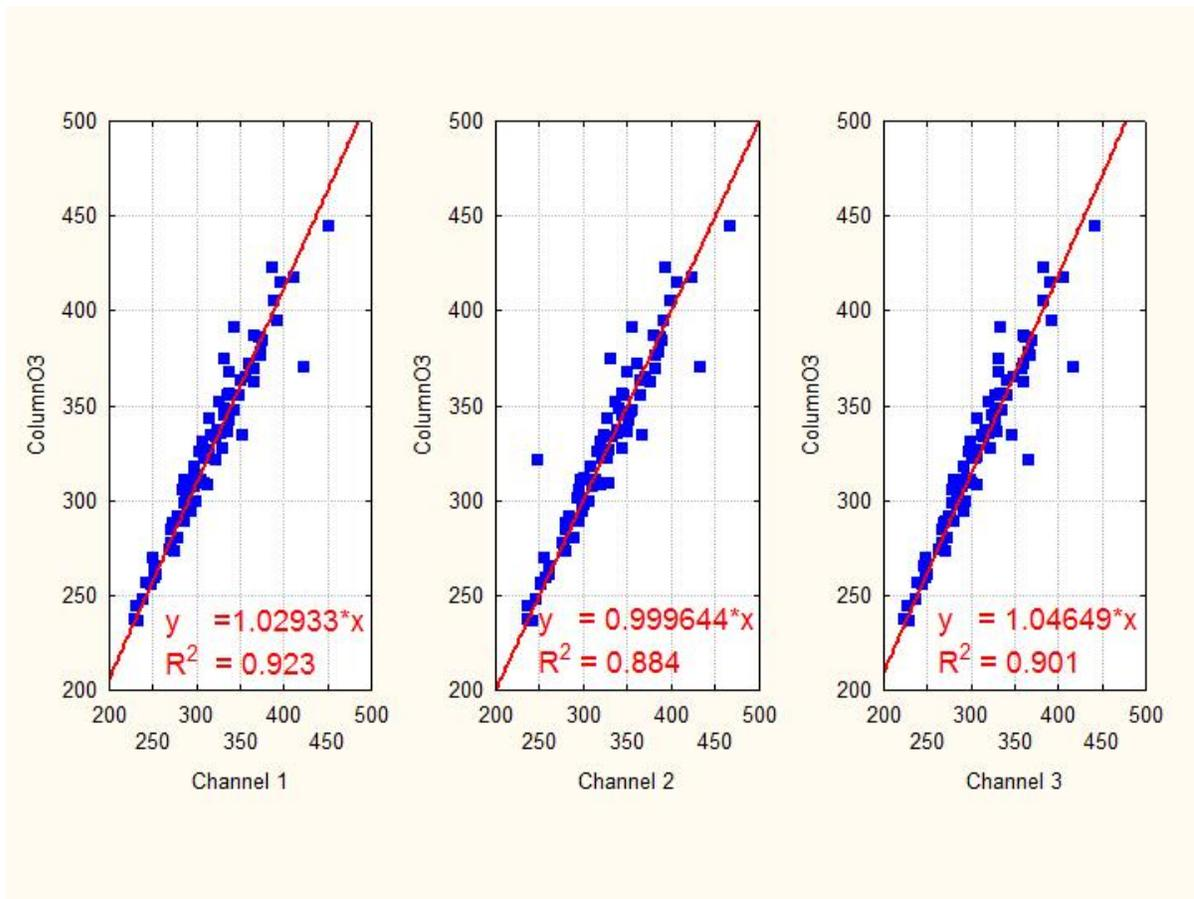
fig. 2 Uccle DS versus the three Microtops channels (N = 84 data points)
