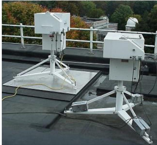
**A comparison of the total ozone measurements done during 2012 with a Microtops II sun photometer and the Uccle Brewer #16 instrument**
